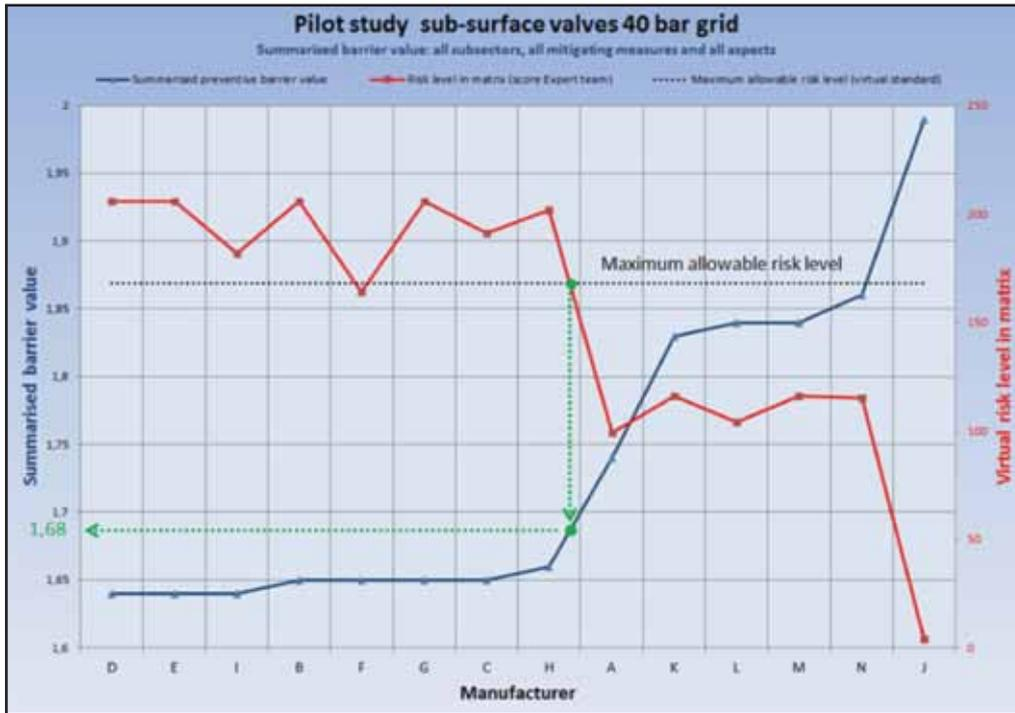
Fig. 13. Relationship between the preventive barrier values of the Bow-tie (blue line) and the virtual risk level (red line).
