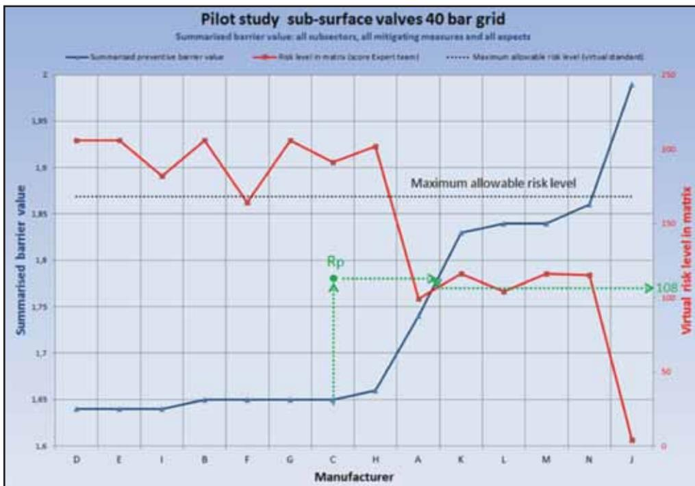
Fig. 14. The increased in value of  $R_p$  for the new design of valve C compared to that of the old design.
