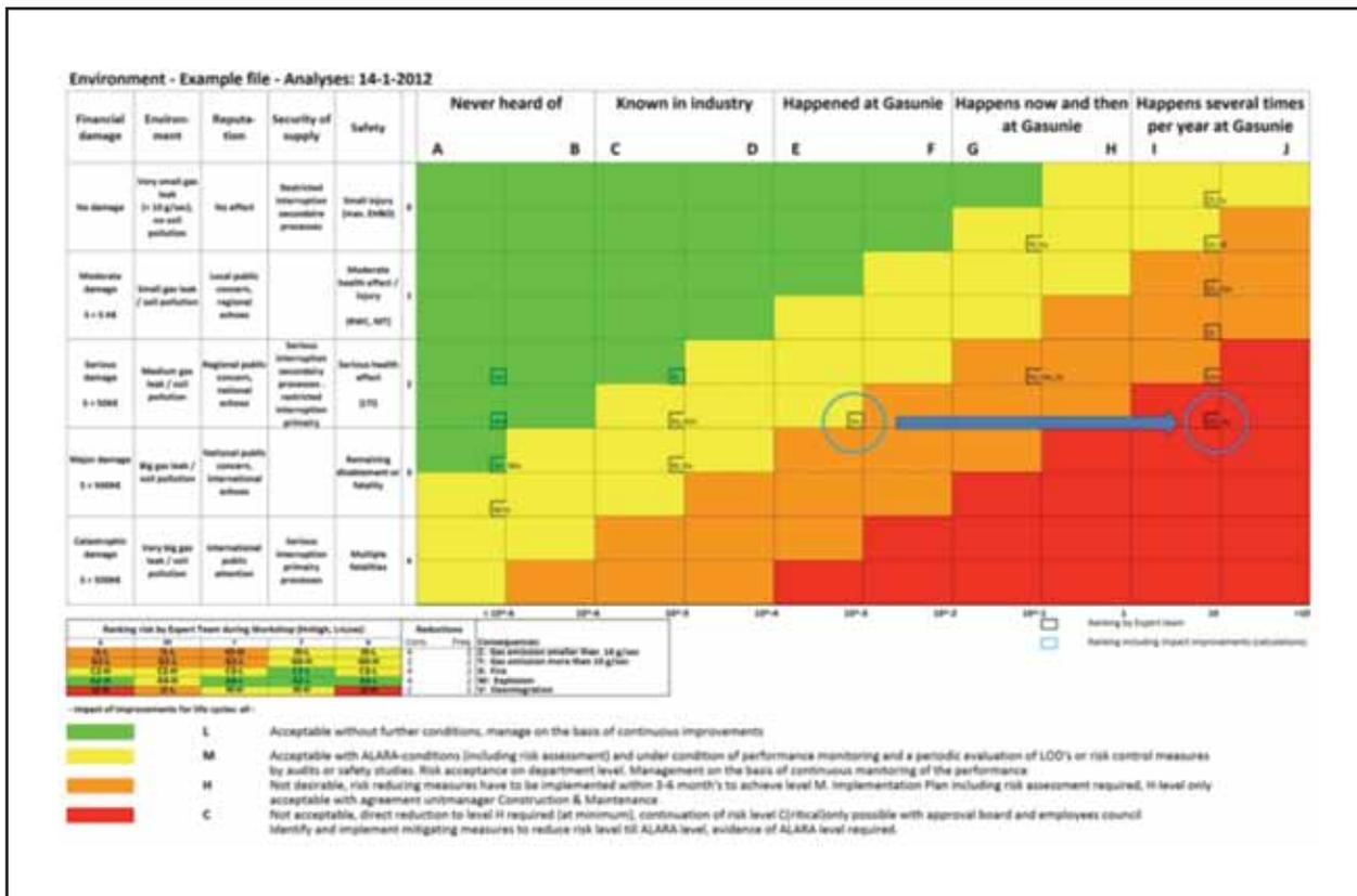
Fig.9. Risk-matrix ranking for one of the 14 valve manufacturers.
