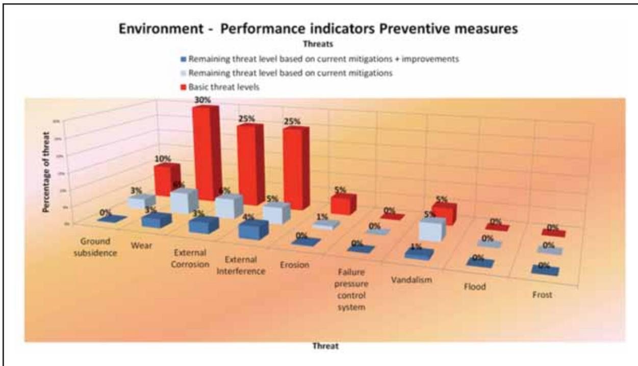
Fig. 11. The main threat to valve integrity.
