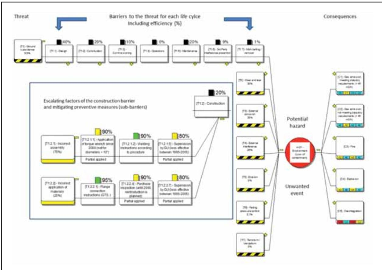
Fig.3. Detail of the Bow-tie diagram for sub-surface valves.
