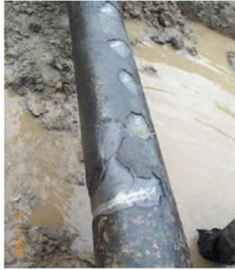
Figure 2. Pipeline coating damage due to excavation.
